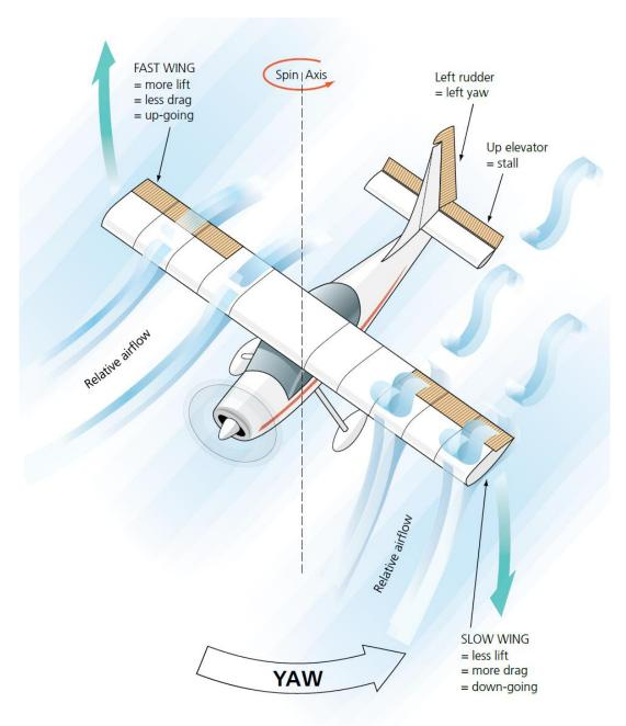
Stall and yaw combine to produce a new axis, the spin axis
