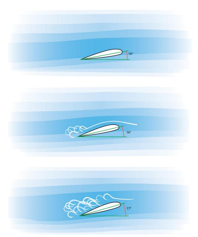
When the stall AoA is reached, the normally streamlined flow of air over the wing becomes turbulent, reducing lift
