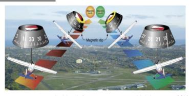
To perform a compass turn, use a controlled bank (e.g. rate one turn which is a turn of 3°/sec or 180° in 60 sec) to change your heading, and then use the compass to confirm your new heading, making small adjustments with a technique called a timed turn.
